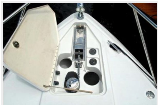
Windlass Anchor Locker
