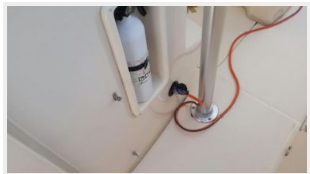
Fire Extinguisher and Battery Charger Outlet
