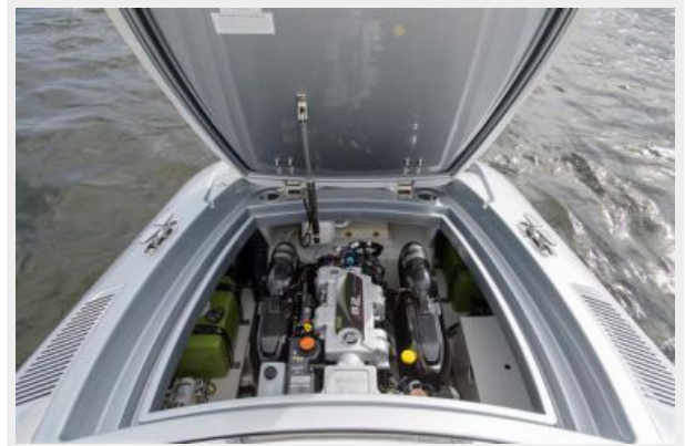
Automatic engine room hatch opening
