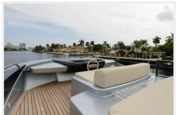
Control station in flybridge
