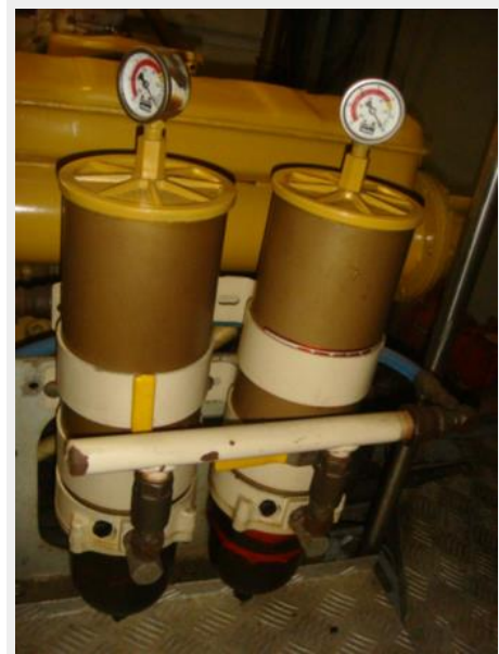
55' Cheoy Lee starboard Racor fuel filters
