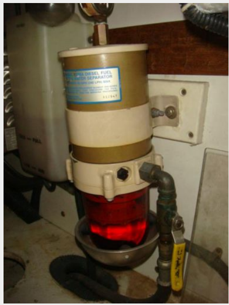
35' Egg Harbor port Racor fuel filter
