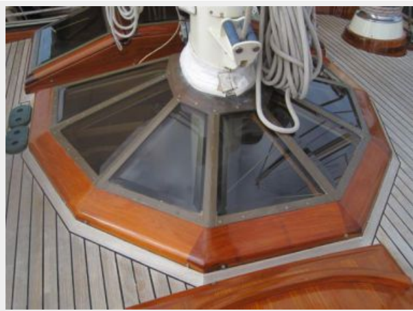
Skylight on deck
