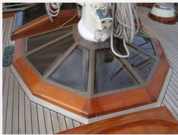
Skylight on deck
