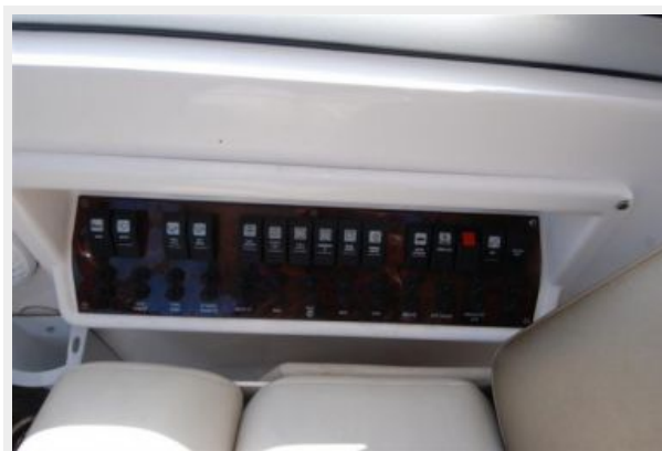
Toggle switches for helm
