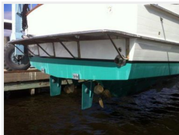
Hull-New Antifouling Paint March 2014
