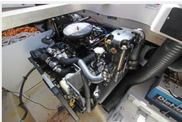
Upgraded 4.3L Mercruiser Engine
