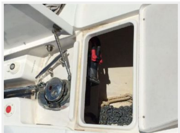
Windlass with foot controls at bow, Anchor line locker
