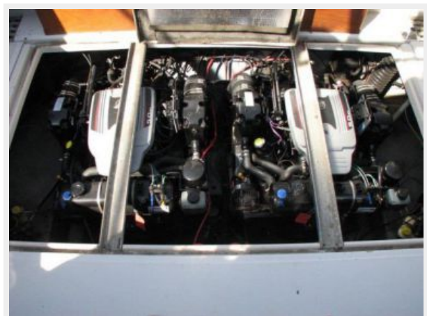
Engine & Mechanical Equipment - Mercruiser 5.0 MPI's
