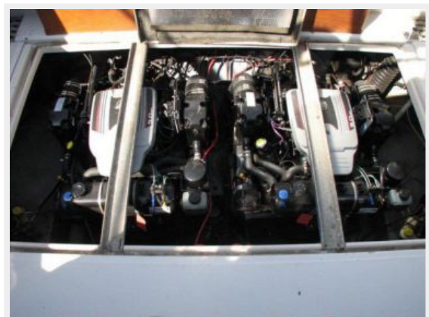
Engine & Mechanical Equipment - Mercruiser 5.0 MPI's
