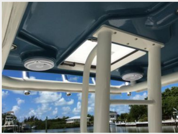
T-Top access to topside
