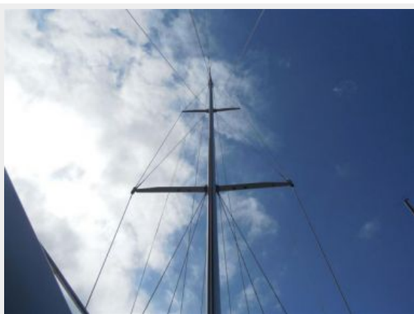
Double Spreader Rig
