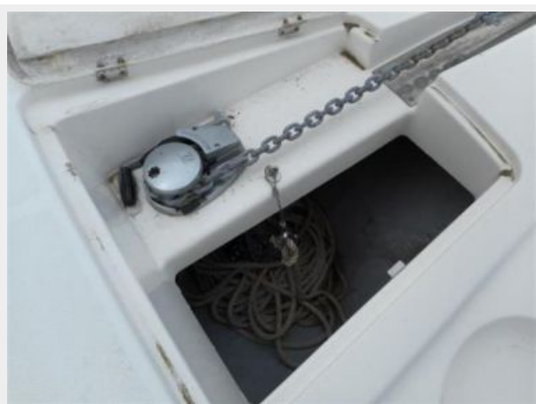
Windlass and anchor locker
