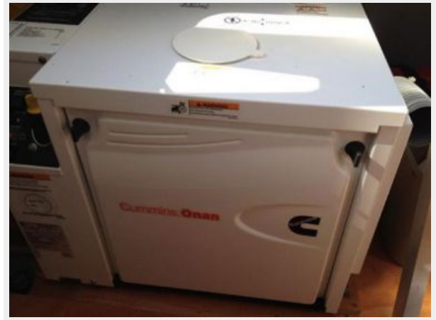
Onan Generator w/sound shield
