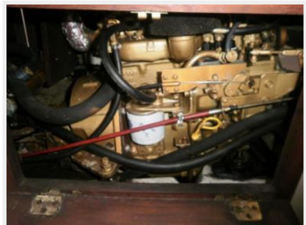
Universal 25hp 3-cylinder "rebuilt" engine
