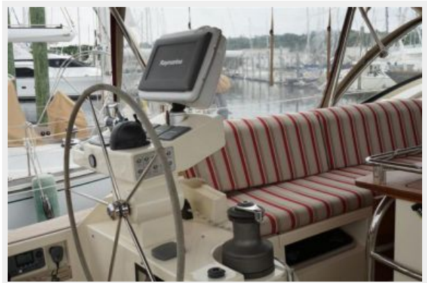
Port Helm Station
