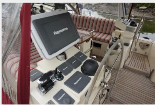
Scanstrut Pods at Helms and Forward
