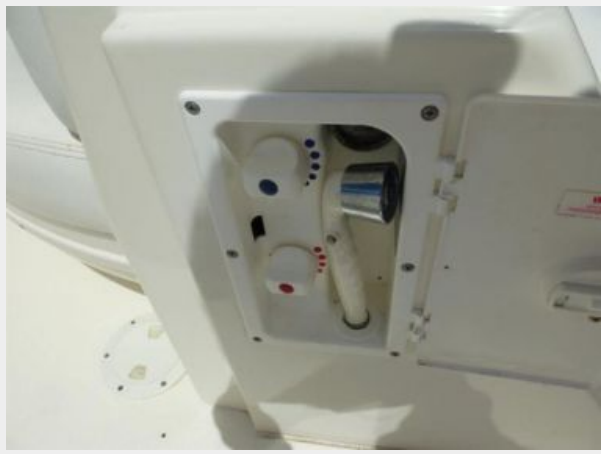
Hot & Cold Fresh Water Shower
