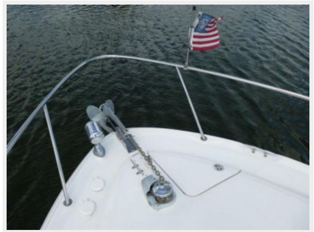
Anchor Windlass & Spotlight
