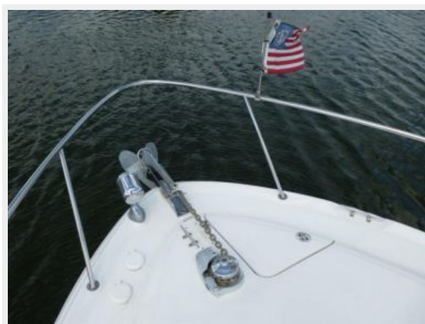
Anchor Windlass & Spotlight
