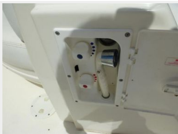
Hot & Cold Fresh Water Shower
