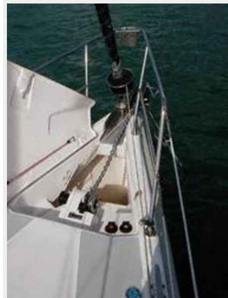
Anchor locker and windlass
