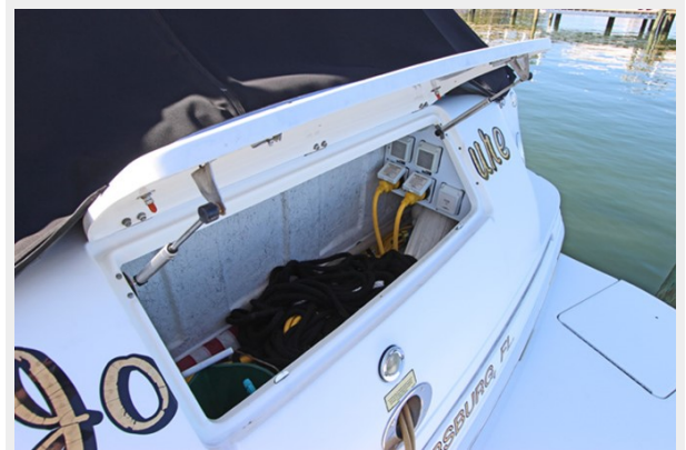
Aft Storage Locker W/2-30 Amp Shore Power Cords
