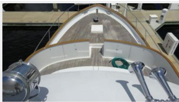
Portugese Bridge Foredeck
