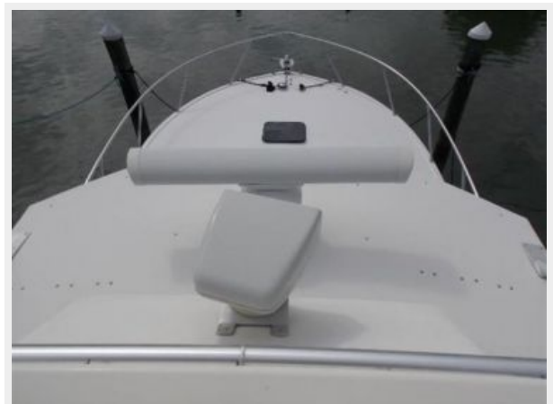
'02 Carolina Classic 35, radar antenna and remote spot light
