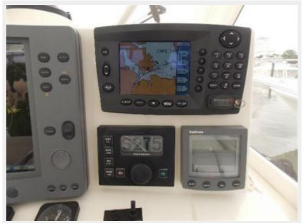
'02 Carolina Classic 35, GPS plotter, Autopilot, Water temp gauge
