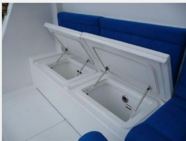
Mezzanine Freezers and Icebox
