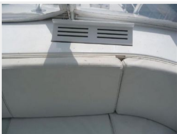
Flybridge AC Vents
