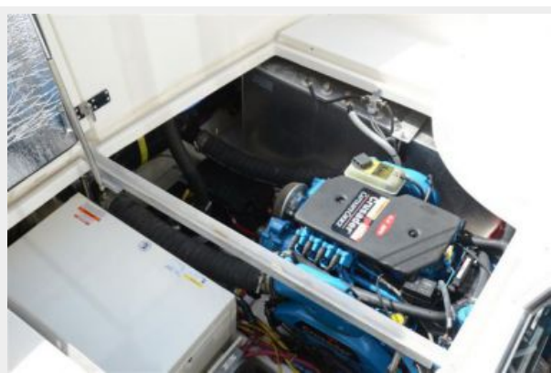
Starboard Motor & Generator
