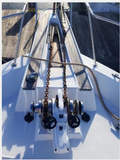
twin anchors and windlass
