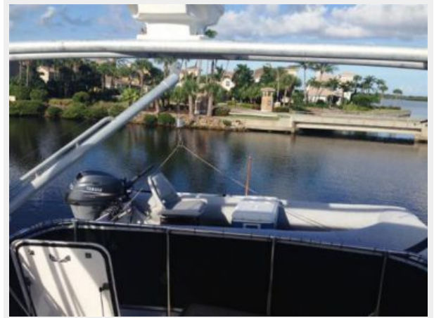
Radar arch and dinghy with davit
