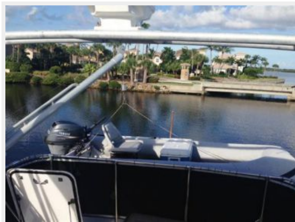
Radar arch and dinghy with davit
