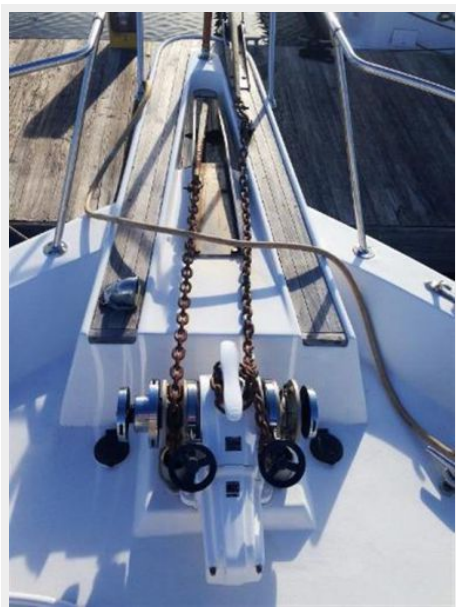
twin anchors and windlass
