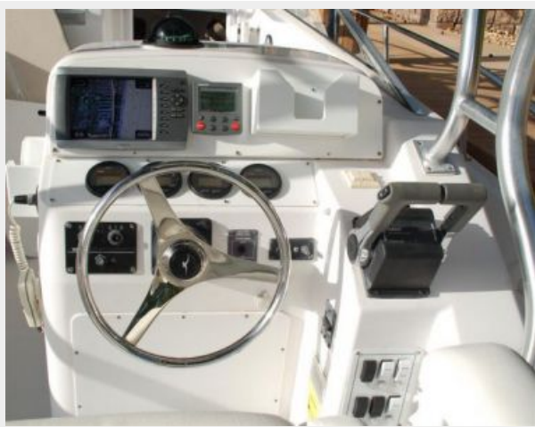
Helm with GPS/Plotter & Autopilot
