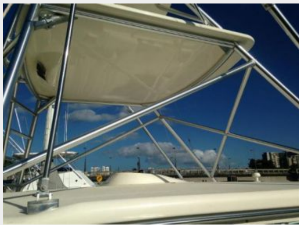
TOWER STANDING PLATFORM AND RADAR SUPPORT
