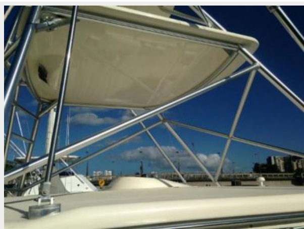
TOWER STANDING PLATFORM AND RADAR SUPPORT
