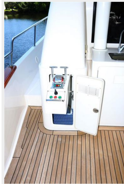
Aft Deck Controls
