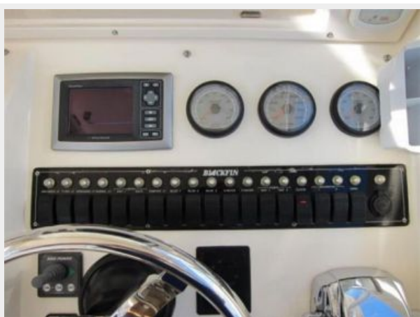
Smartcraft Gauges, switch panel
