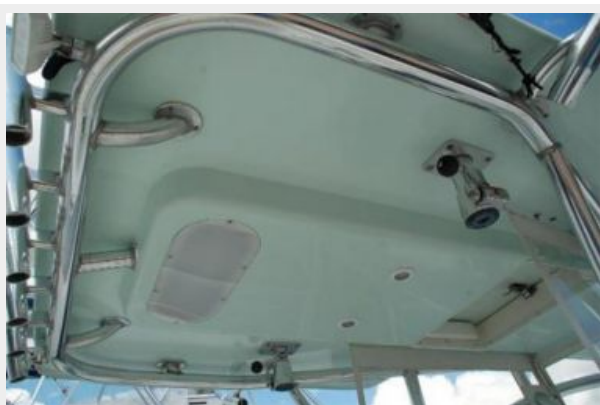
Underside of hardtop, gelcoat matches hull
