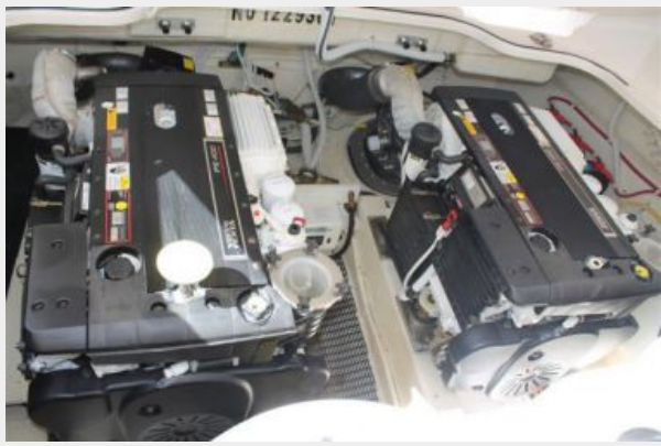
Twin Volvo IPS-400 Diesel Power
