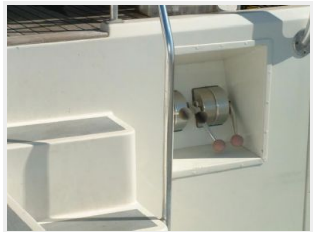
Cockpit level docking station
