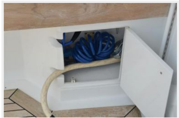
58 Davis Cablemaster Port
