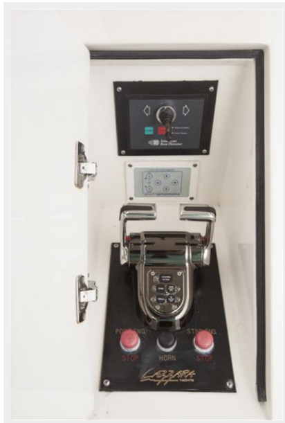
Aft Control Station
