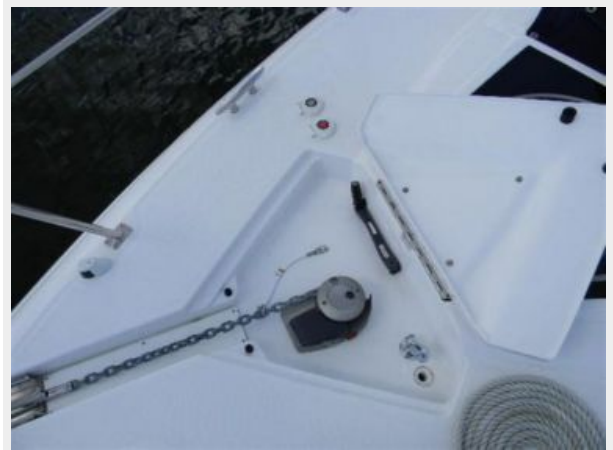
Recessed Windlass, Anchor, Line & Chain
