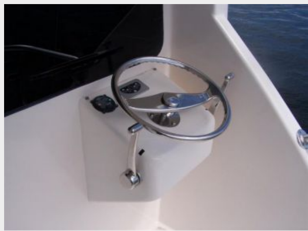
Aft Bridge Station
