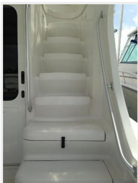
Molded Fiberglass Steps to Bridge
