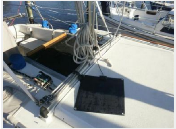
Small Solar Panel Keeps Batteries Topped off
