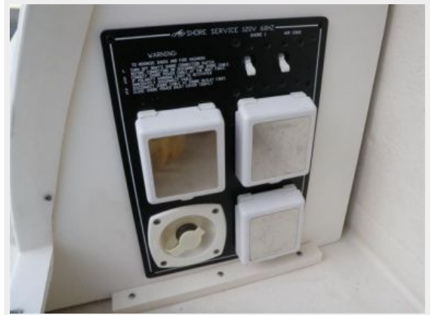
Shore power connections
