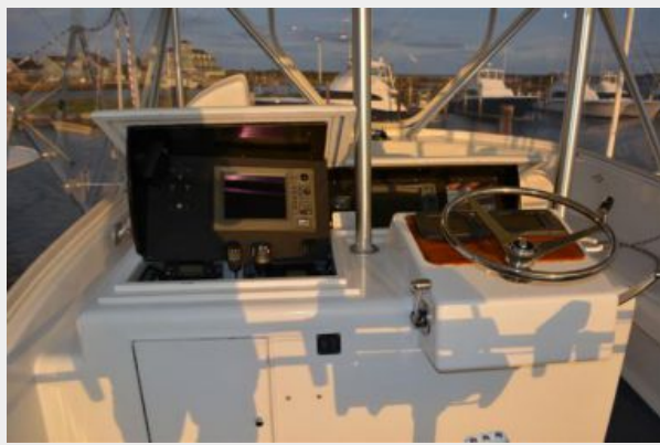
Actuated electronics panel up
