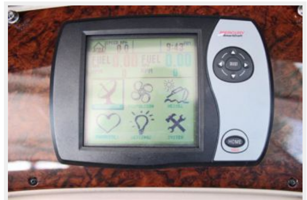
Smartcraft Engine Monitoring System
