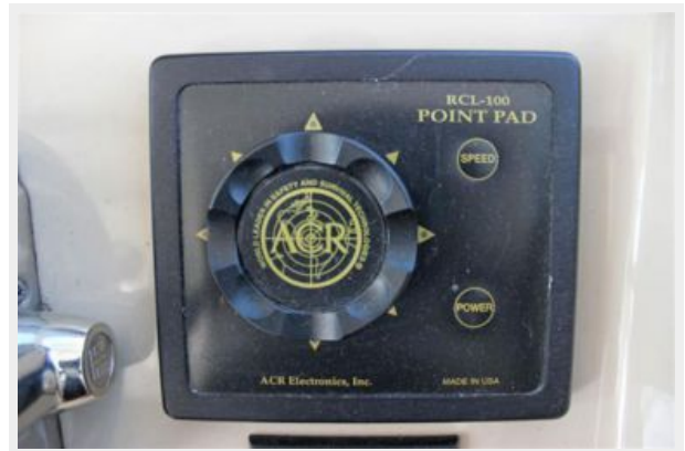
ACR Point Pad Control For Bow Spotlight
